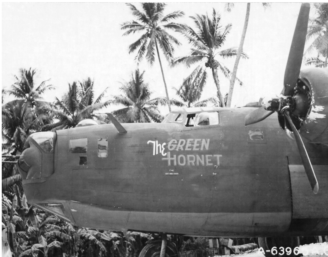
“THE GREEN HORNET” on Funafuti (18-23 April 1943) shows tail turret moved to nose position. US AAF photo.
