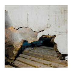
This public-domain NASA image pinpoints the place where the accident causing the loss of *Challenger* began. NASA describes the image with these words: "Shown here is an interior view of the scorched hole in Space Shuttle *Challenger's* right Solid Rocket Motor. The tapered edges along the hole indicate the inside to outside path of the fire that led to the accident." Click on the image for a full-page view.
