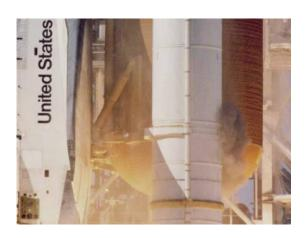
This NASA image depicts the first evidence of black smoke from the lowermost joint of the right-hand Solid Rocket Booster (SRB) on the day STS 51-L (the official designation of *Challenger's* final mission) left the launchpad. The image shows the condition of the aft field joint milliseconds after liftoff.
