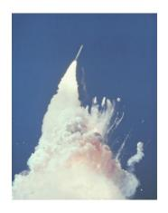
In this NASA image, we see the Challenger exploding on January 28, 1986. All seven members of the crew died. NASA's Technical Report describes this image: "At about 76 seconds, fragments of the Orbiter can be seen tumbling against a background of fire, smoke and vaporized propellants from the External Tank. The left Solid Rocket Booster (SRB) flys rampant, still thrusting." Click on the image for a better view.
