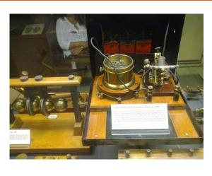
Part of Marconi's famous invention - "the wireless" - which allowed people to transmit and receive messages via radio waves. Here we see the actual <u>coherer (receiver)</u> which Marconi used, in 1896, to describe the power of his invention. It is currently maintained at the Oxford Museum of the History of Science. *Titanic* used a Marconi wireless. Photo by Ozeye, online via Wikimedia Commons. Image license: <u>CC BY-SA 3.0</u>
