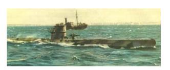
This image depicts U-760 (a Type VIIC U-Boat) at sea. Because this type of vessel (in the foreground) is a submarine, it does not have much freeboard above the water. Image online, courtesy U-Boat.net.
