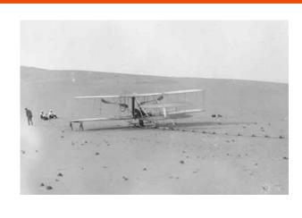
This image depicts a powered plane which the Wright Brothers called "Flyer 3" which first flew in 1905. The photo has this description, <u>from the Library of Congress</u>: "The remodeled 1905 Wright machine, altered to allow the operator to assume a sitting position and to provide a seat for a passenger, on the launching track at Kill Devil Hills. This is apparently the only photograph of this machine taken by the Wright brothers in 1908."
