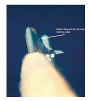
Unexpected Trouble - Debris Near the Orbiter's Left Wing
