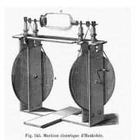
Hauksbee Electrostatic Generator and Neon Light Image, from a French-langage work, depicting Hauksbee's modified electrostatic generator as it appeared, circa 1706. View this asset at: http://www.awesomestories.com/asset/view/Hauksbee-Electrostatic-Generator-and-Neon-Light
