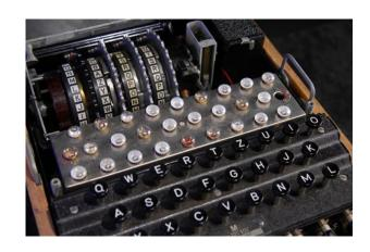
This photo of a 4-rotor Enigma machine gives us a view of the rotors, the lamp board, the keyboard and a small view of the plugboard. Online via the U.S. Air Force Network Integration Center. Photo credit: AF ISR Agency History Office. Click on the image for a better view.
